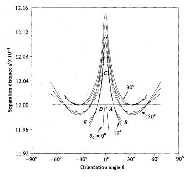
FIGURE 16. Trajectories for a neutrally buoyant slender body in a simple shear flow  $\hat{U}_2 = \Gamma_{13} x_3 e_1$  in terms of the separation distance d and the orientation angle  $\theta$ ;  $\phi_0 = 30^\circ$ ,  $\theta_0 = -30^\circ$ ,  $0^\circ$ ,  $10^\circ$ ,  $50^\circ$ ,  $\kappa = 20$ , S(x) = 0,  $x_p^0 = (0, 0, -1.2)$ : ----,  $\lambda = \infty$ ; -----, 1; ----,  $\lambda = 0$ ; -----, unbounded-fluid case.
