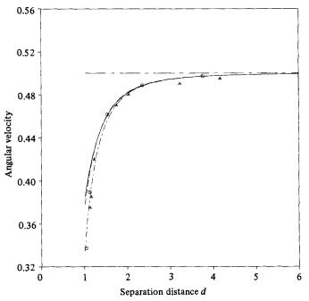
FIGURE 12. Dimensionless angular velocity  $-\Omega_2/\Gamma_{13}$  as a function of the dimensionless distance d between the sphere centre and the interface;  $U_2 = \Gamma_{13} x_3 e_1$ : ...,  $\lambda = \infty$ ; ..., 1; ...,  $\lambda = 0$ ; ..., 1; ...,  $\lambda = 0$ ; ..., and  $\lambda = 0$ ; ...,  $\lambda = 0$ ; ...,
