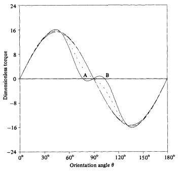
FIGURE 7. Dimensionless torque  $T_2/\epsilon\mu_2 El^3$  of (24b) as a function of the orientation angle  $\theta$ ;  $\hat{U}_2 = \boldsymbol{E} \cdot (\boldsymbol{x} - \boldsymbol{x}_p), \epsilon = 0.1887, S(x) = \frac{1}{2} \ln [1 - (x/l)^2], d = 1.01:$ ,  $\lambda = \infty$ ; ..., 1; ..., 0, ..., unbounded-fluid case.
