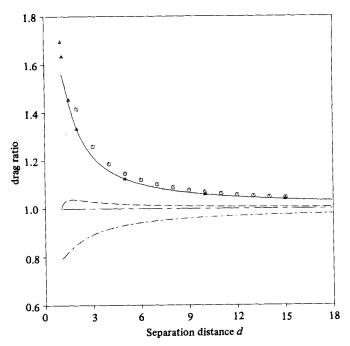
FIGURE 3. Drag ratio relative to the drag in an unbounded fluid as a function of the dimensionless distance d between the sphere centre and the interface;  $\hat{U}_2 = \Gamma_{13} x_3 e_1$ :  $\dots$ ,  $\lambda = \infty$ ;  $\dots$ , 1;  $\dots$ , 0;  $\Delta$ , corresponding exact-solution results of Goren & O'Neill (1971);  $\bigcirc$ , data of Wakiya (1957) for two parallel plates.
