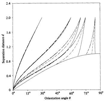
FIGURE 13. Trajectories for a neutrally buoyant slender body in a pure straining flow  $U_2 = \mathbf{E} \cdot \mathbf{x}$ , interms of the  $\theta$  and  $d; \phi_0 = 0^\circ, \theta_0 = 0^\circ, 30^\circ, 60^\circ, 70^\circ, 75^\circ, 85^\circ$  and  $90^\circ, \epsilon = 0.1883, S(x) = \frac{1}{2} \ln [1 - (x/l)^2];$ ....,  $\lambda = \infty;$  ....,  $\lambda = 1;$  ...., 0, ...., unbounded-fluid case.
