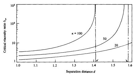
FIGURE 8. Critical viscosity ratio  $\lambda_{er}$ , as a function of the separation distance d for aspect ratios  $\kappa = 20, 50$  and  $100; \hat{U}_2 = \boldsymbol{E} \cdot (\boldsymbol{x} - \boldsymbol{x}_p)$  and  $S(x) = \frac{1}{2} \ln [1 - (x/l)^2]$ .
