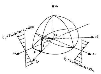
FIGURE 4. Orientation of a slender body in a simple shearing flow with the origin at the body centre. The  $(x_1, x_2)$ -plane is parallel to the interface.
