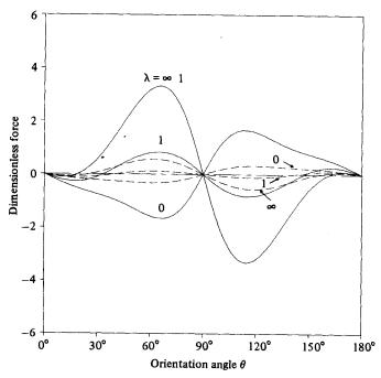
FIGURE 5. Dimensionless force,  $F_1/\epsilon^2 \mu_2 El^2$  of (24*a*) as a function of the orientation angle  $\theta$ ;  $\hat{U}_2 = \boldsymbol{E} \cdot (\boldsymbol{x} - \boldsymbol{x}_p), \ \epsilon = 0.1887, \ S(x) = \frac{1}{2} \ln [1 - (x/l)^2]; \ \dots, \ d = 1.01; \ \dots, \ 2.0; \ \dots, \ n$ bounded-fluid case.
