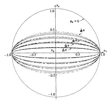
FIGURE 15. Orbital trajectories as obtained by the projection of the end of the particle onto the plane of the shear flow  $\hat{U}_2 = \Gamma_{13} x_3 e_1$ ;  $\phi_0 = 0^\circ$ ,  $\frac{1}{48}\pi$ ,  $\frac{1}{36}\pi$ ,  $\frac{1}{24}\pi$  and  $\frac{1}{12}\pi$ ,  $\theta_0 = 0^\circ$ ,  $\kappa = 20$ , S(x) = 0,  $x_p^0 = (0, 0, -1.2)$ : ...,  $\lambda = \infty$ ; ..., 1; ..., 0; ..., 0; ..., unbounded-fluid case.
