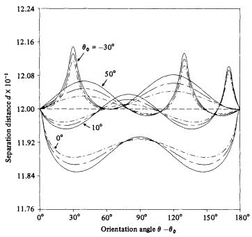
FIGURE 14. Trajectories for a neutrally buoyant slender body in a simple shear flow  $U_2 = \Gamma_{13} x_3 e_1$ in terms of the separation distance d and the orientation angle  $\theta$ ;  $\phi_0 = 0^\circ$ ,  $\theta_0 = -30^\circ$ ,  $0^\circ$ ,  $10^\circ$ ,  $50^\circ$ ,  $\kappa = 20$ , S(x) = 0,  $x_p^0 = (0, 0, -1.2)$ : ---,  $\lambda = \infty$ , ----, 1; ---, 0, ----, unbounded-fluid case.
